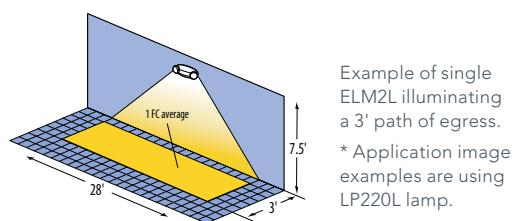
Also meets the additional illumination requirements of NFPA 101: 1FC minimum and max/min ratio of 40:1.
