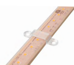
Mounting Clips – Provide secure attachment to a variety of surfaces when placed at 1-foot intervals. The back of luminaires features 3M adhesive strips to maintain positioning while installing clips.
