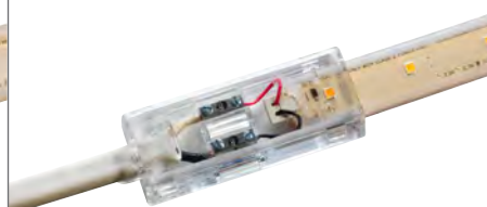
Terminal Block – Accepts 14-22 AWG wire, allowing power supply to be remotely mounted up to 100 feet away.
